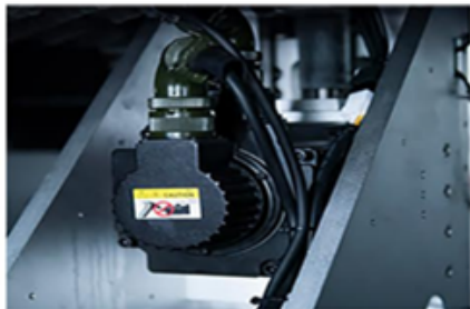
1.5 KW head-driven motor
